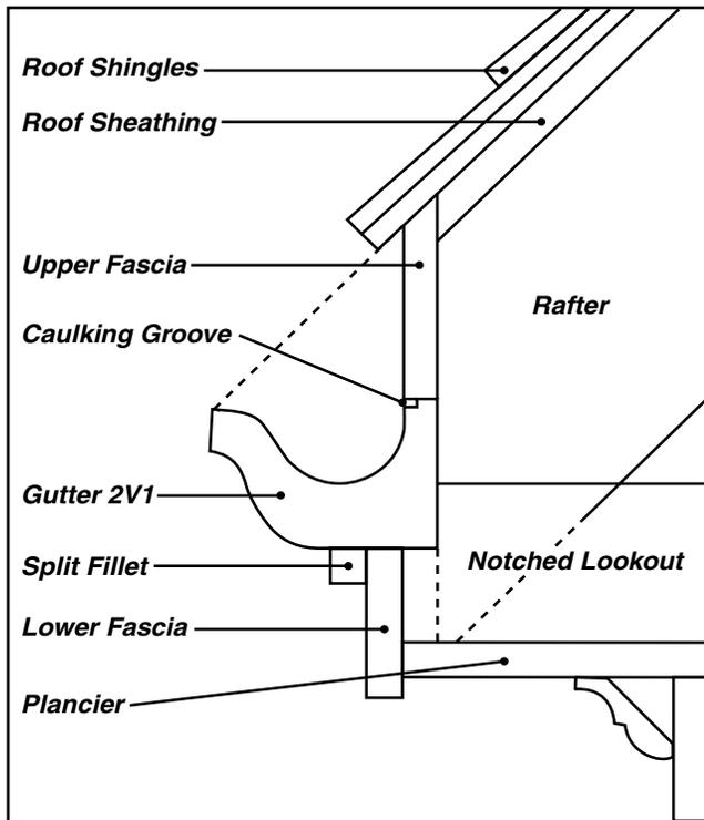
Figure 4: Section Through Eaves Showing Boston Pattern Milled Wood Gutter
