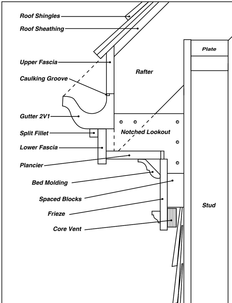
Figure 7: Suggested Detail Of Traditional Gutter Cornice Modified To Incorporate Continuous Eaves Vent Strip.
