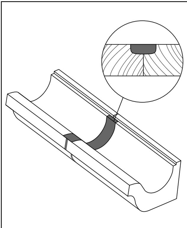
**Figure 7:** Gutter Joint Detail Using Urethane Caulk Web
