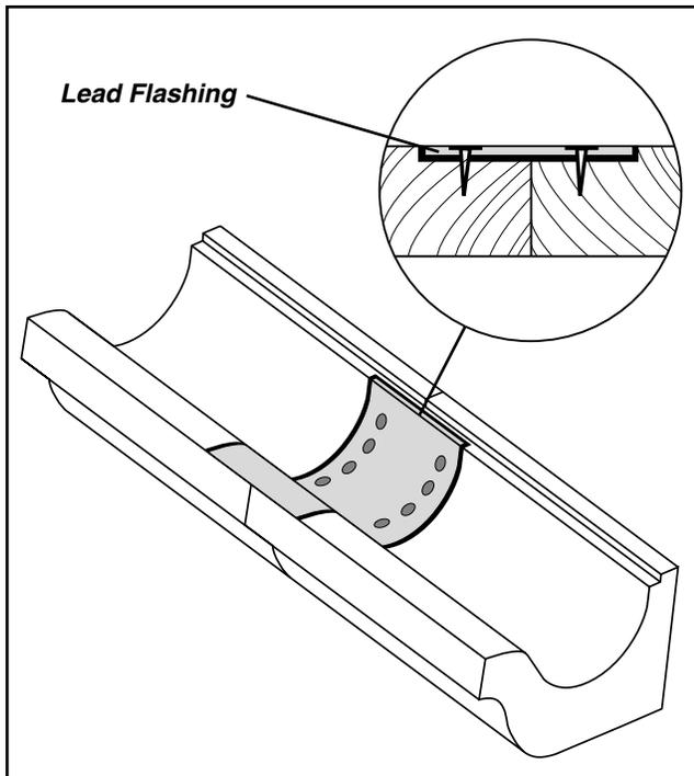
**Figure 6:** Gutter Joint Showing Traditional Lead Web Set in Asphalt Flashing Cement
