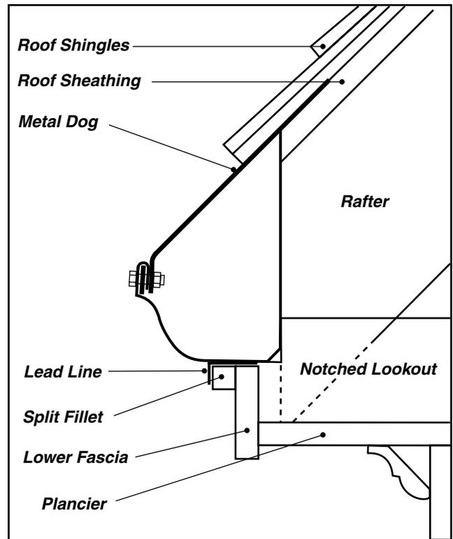
Figure 3: Section Through Sheet Metal Gutter - Victorian Period
