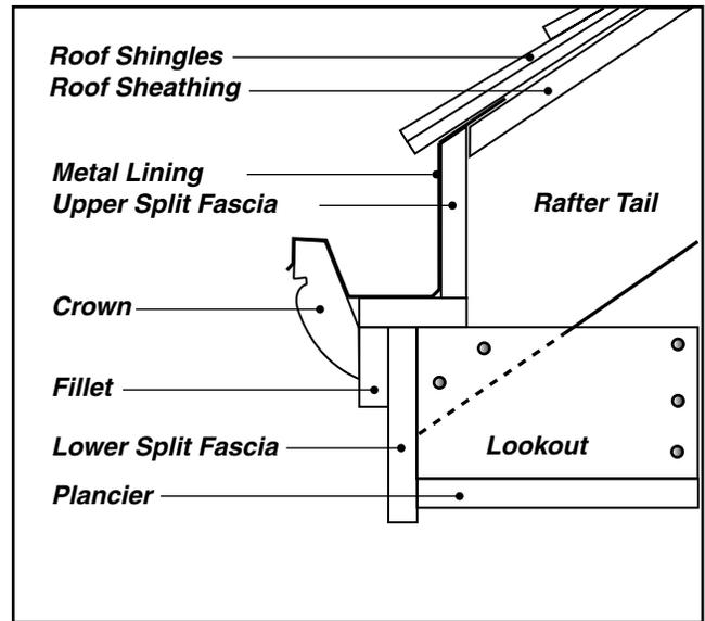
Figure 2: Section Through Metal Lined Gutter Greek Revival Period
