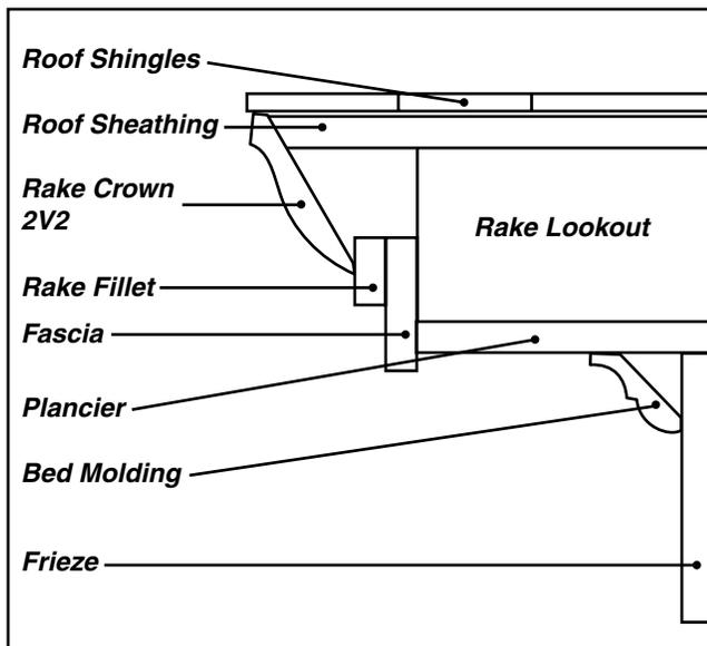
Figure 5: Section Through Raking Cornice Showing Boston Pattern Rake Crown Configured For Rake Miter
