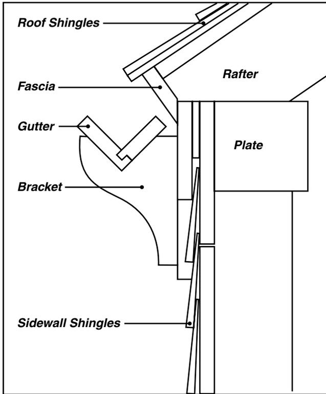
Figure 1: Section Through "V" Trough Gutter Colonial Period
